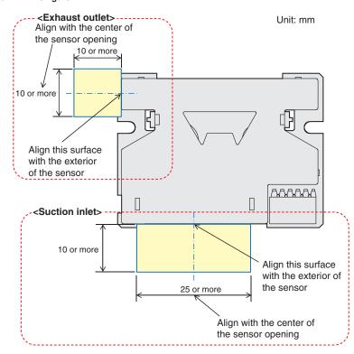
Note1: Ensure that the suction inlet and exhaust outlet are as close to the sensor case in the forward and rear directions as possible
