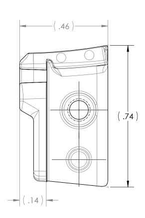
NOTE: TIE TAIL LENGTH INCREASED BY APPROXIMATLY 3MM OVER STANDARD NOSEPIECE
