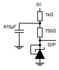
**Test Circuit for Input Noise Voltage**
