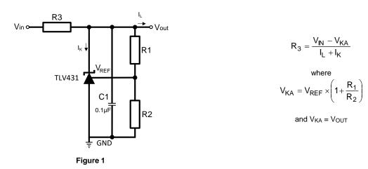
The values of R1 and R2 should be large enough so that the current flowing through them is much smaller than the current through R3, yet not too large that the voltage drop across them causes I<sub>REF</sub> to affect the reference accuracy.
