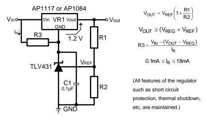
Figure 7. Adjustable Linear Voltage Regulator
