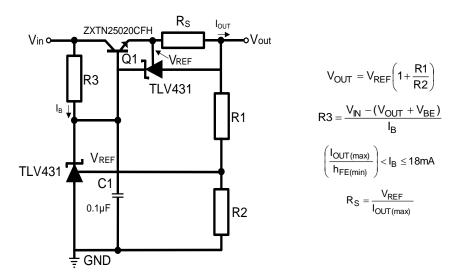
Figure 5. Series Regulator with Current Limit
