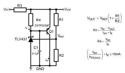
Figure 3. High-Current Shunt Regulator
