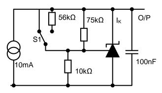
**Test Circuit for VREF Measurement**
