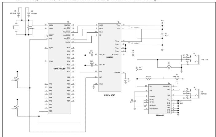
FIGURE 9: APPLICATION EXAMPLE USING SPI
