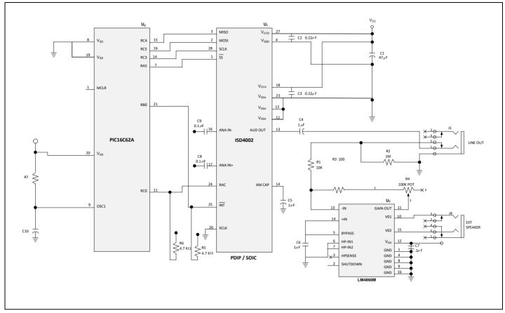
FIGURE 10: APPLICATION EXAMPLE USING MICROWIRE
