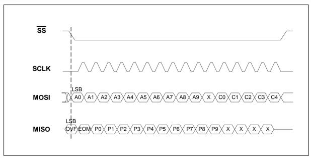
**FIGURE 7: 16-BIT COMMAND FORMAT**
