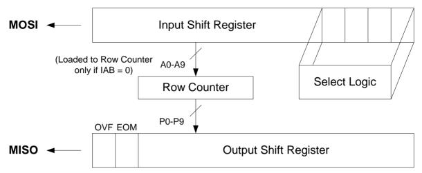
FIGURE 3: SPI INTERFACE SIMPLIFIED BLOCK DIAGRAM
