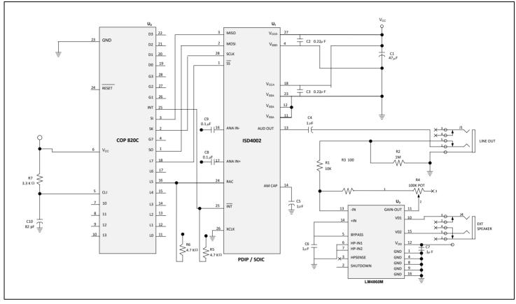
FIGURE 11: APPLICATION EXAMPLE USING SPI PORT ON MICROCONTROLLER
