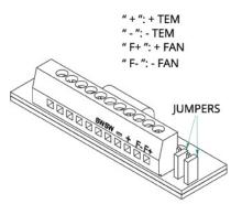
To use a separate supply for TEMs and FANs: Mount jumpers to not short-cut the pin pairs.
