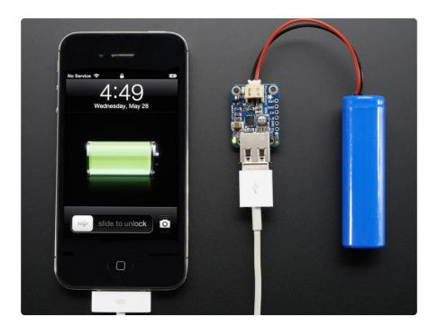
Great for powering your robot, Arduino project, single-board-computer such as Raspberry Pi or BeagleBone! Each order comes with one fully assembled and tested PCB and a loose USB A jack. If you are powering your project from USB, solder the USB A jack in (a 3-minute soldering task). If you would like to use a terminal block, pick up a 3.5mm 2pin block here () and solder to the output spot where the USB jack would go. Or dont solder anything in for a more compact power pack.
