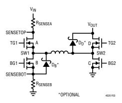
Figure 3. Converter Switch Diagram
