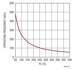
Figure 7. R<sub>T</sub> vs Operating Frequency
