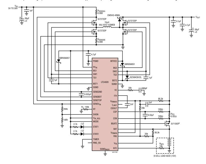
15V to 55V to 6-cell Li-lon PowerPath charger/system supply. 6A inductor current limit with 2.5A battery charge current limit. Instant-on functionality for battery voltages below 20.4V, 24V charge termination voltage, and 26.4V maximum output voltage. Status pins light LEDs for visible charge-state monitoring
