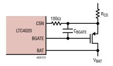
Figure 21. Instant-On/Ideal Diode Compensation
