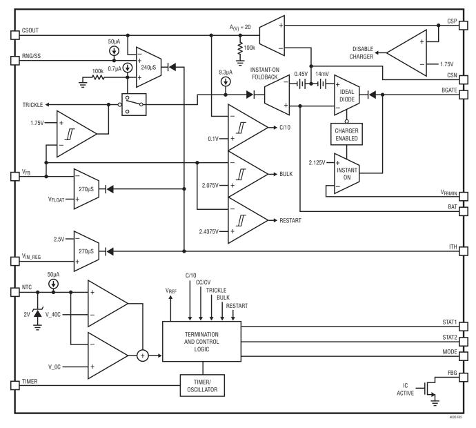
Figure 2. Battery Charger Block Diagram
