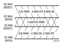
Figure 4. Operating Regions vs Duty Cycle (DC)
