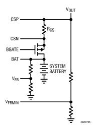
Figure 5. Battery Charger PowerPath Diagram
