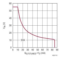
Figure 10. INTV<sub>CC</sub> Pass Element SOA (Safe Operating Area)
