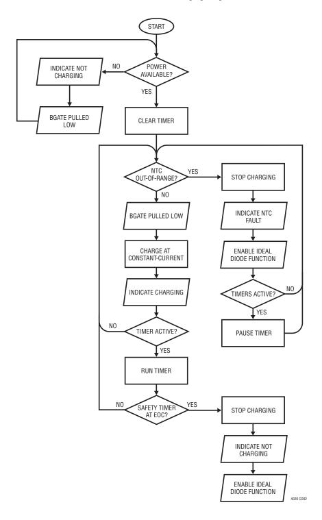
5V to 30V to 6-cell lead-acid PowerPath charger/system supply. 6A inductor current limit with 2.5A battery charge current limit. Instant-on functionality incorporated for battery voltages below 12.25V, 14.4V absorption voltage, 13.3V float voltage, and 15.6V maximum output voltage (Instant-On and NTC fault only). Status pins light LEDs for visible charge-state monitoring
