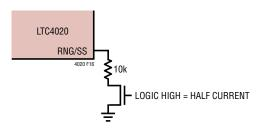
Figure 16. Using the RNG/SS Pin for Digital Control of Maximum Charge Current
